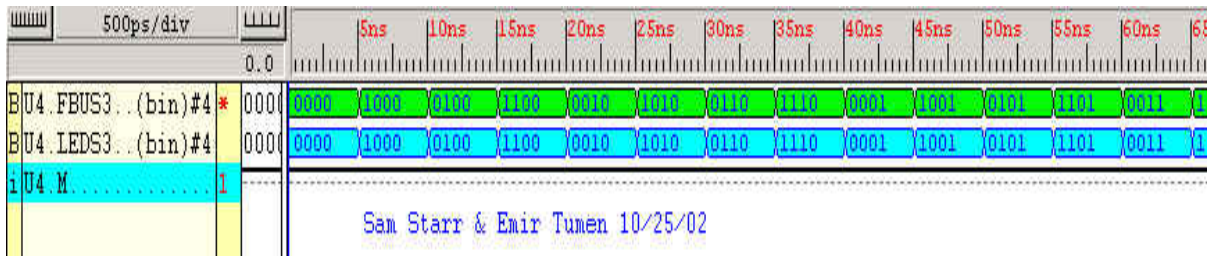
Figure 18: Functional Simulation of LED Decoder
